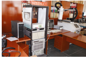
Electrical characterization: 4200SCS system (Keithley, UK): Voltage CC<100V, Current CC<1A; Impulses: analogical signal 30V, <40MHz; Measurements: Voltage 0.5 \mu V, Current 1 fA.
